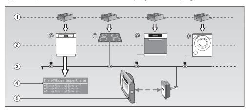
These instructions are for a communication enabled dishwasher ② that can be linked into the Miele@home system via a communication module ① (optional accessory).
